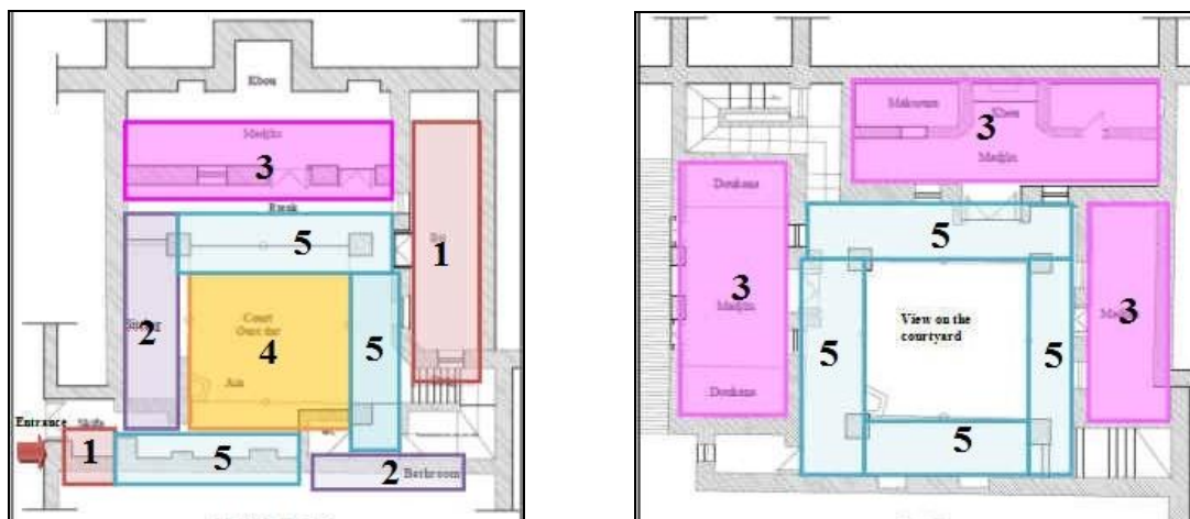
Figure 2 Typical layout of a courtyard house in the City of Constantine, Algeria (ground floor left, first floor right) Key: 1 = Public (Bit, skiffa); 2 = Semi public (Services); 3 = Private (Female and family living, or bedroom); 4 = Open space (Courtyard); 5 = Transitional spaces (Riwak).
