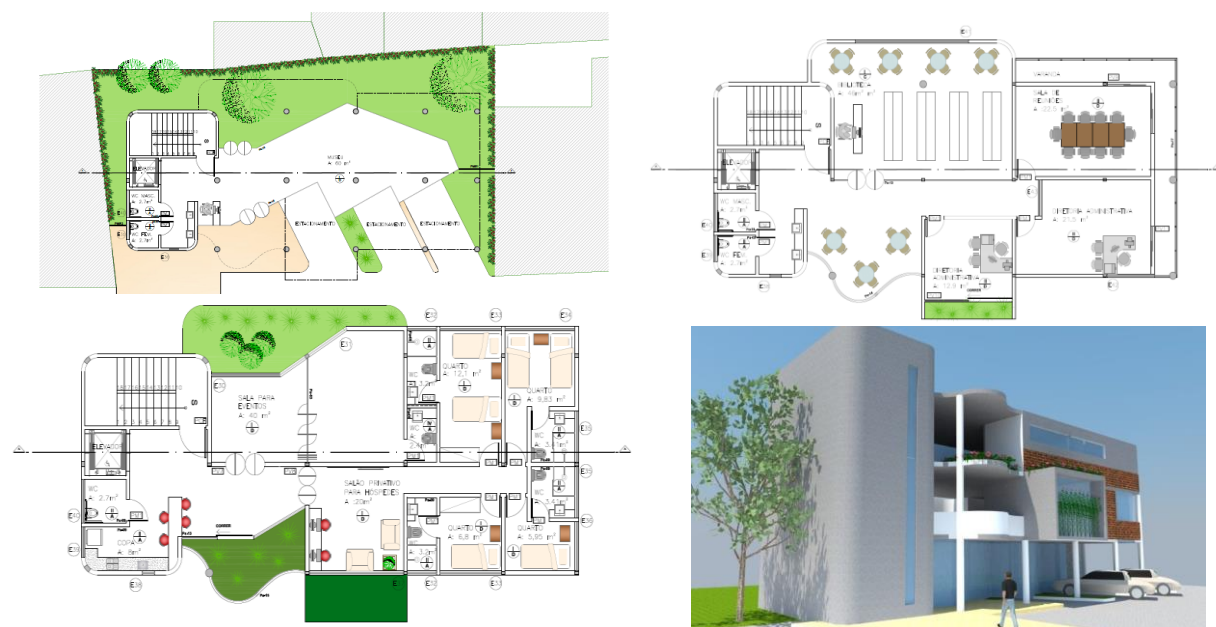
Figure 4 (a) Floor plan of ground level, (b) Floor plan of the first level, (c) floor plan of the second level, and (d) annex building facade.
