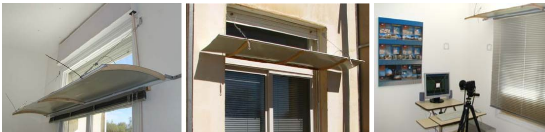
Figure 1 Light shelf installed for the experiment, seen from interior (left) and exterior (middle); setup for HDR photography used to establish luminance (right).
